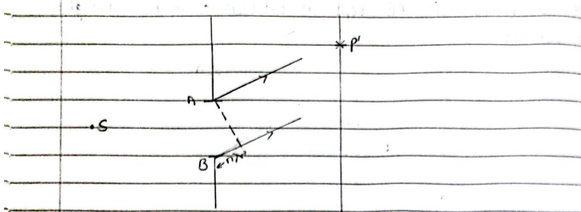
Consider any point  $P'$  on the screen. The point  $P'$  will be dark if the path difference between  $AP'$  and  $BP'$  is equal to  $n\lambda$ .
