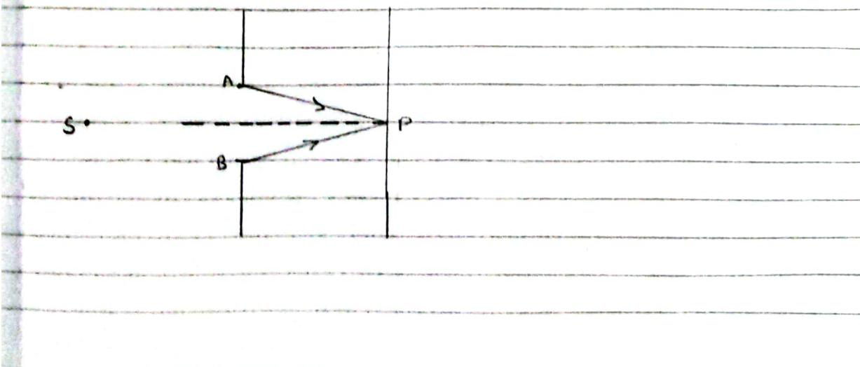
Let P be the midpoint of the screen, then the path difference between 2 waves reaching the point P from A and B will be 0.
