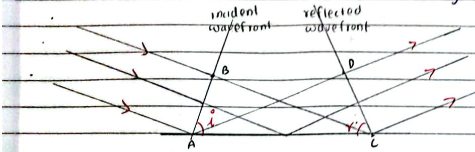
In the figure, <sup>AB is</sup> the incident wavefront and CD is the reflected wavefront.  $i$  is the angle of incidence and  $r$  is the angle of reflection.
