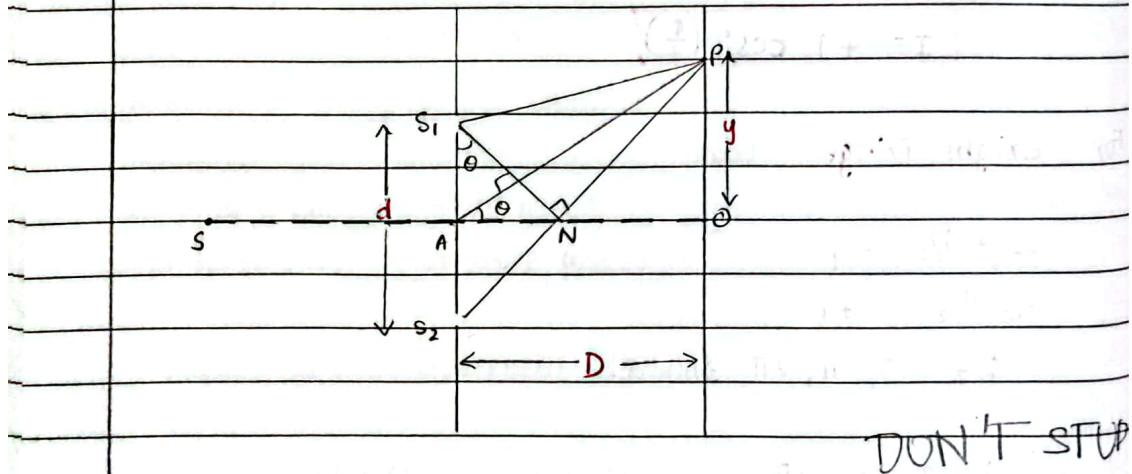
Consider a YDSE setup consisting of 2 slits  $s_1$  and  $s_2$  separated by a small distance 'd'. The screen is placed at a distance 'D' from the slits. P is a point on the screen at a distance 'y' from the central bright fringe.
