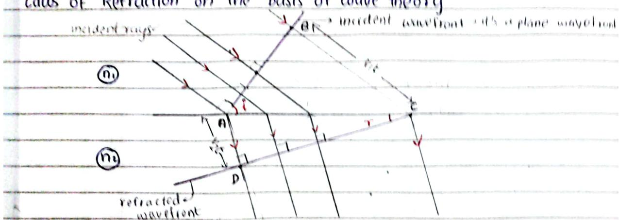
In figure, AB is the incident wavefront in a medium of refractive index  $n_1$  and CD is the refracted wavefront in a medium of refractive index  $n_2$ .  $i$  is the angle of incidence and  $r$  is the angle of refraction.
