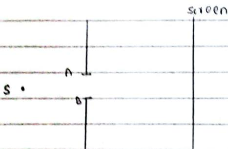
On the screen, one can observe alternate bright and dark rings with a bright spot at the centre.
