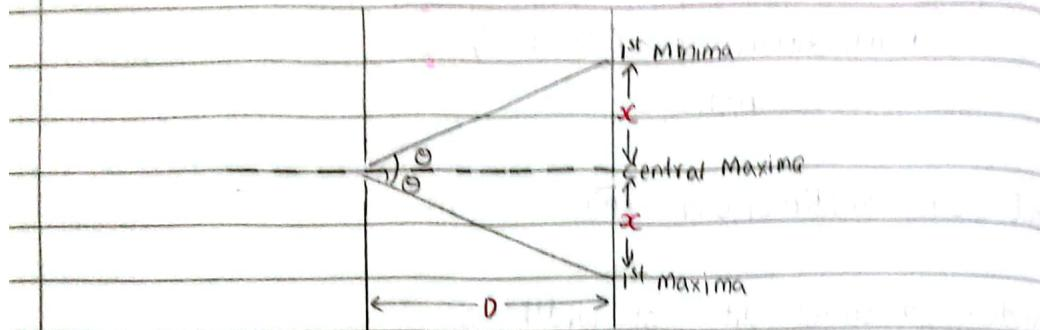
Consider the formation of a single slit diffraction pattern. Let 'a' be the width of the slit and 'D' be the distance between the slit and screen.
